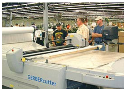
Figure 30: Automated Fabric Cutter in Use at MARC Custom Medical Products
